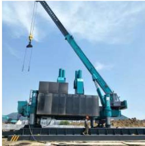
Gambar 2.4: Alat Hydraulic Static Pile Driver (HSPD) Kapasitas 420 Ton (Penelitian, 2021)
