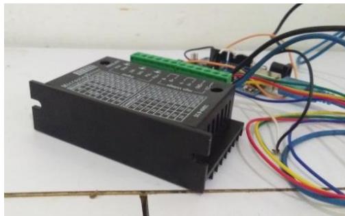
Gambar 3.18. Driver Motor TB6600
