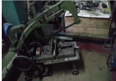
Gambar 4.28 Memotong Besi Bulat
