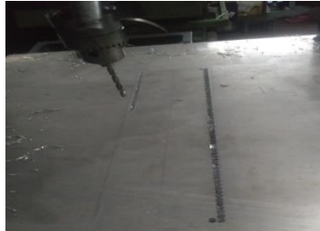
Gambar 4.49 Melubangi Base Turbin
