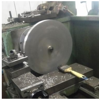
Gambar 4.34 Meletakkan Runner dicark Mesin Bubut
