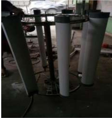
**Gambar: 2.5 Kincir angin sumbu vertikal model sarvonius**
