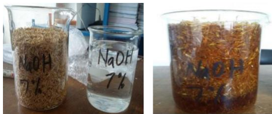
Gambar 2.1. preparasi larutan NaOH 7% (Suartama dkk,2016).
