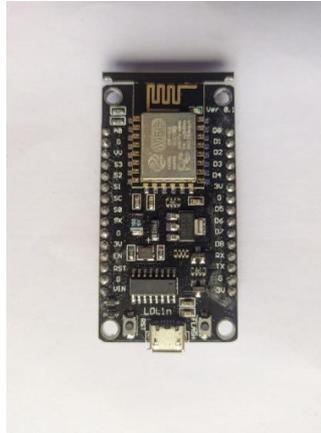
Gambar 2.11 Modul Wi-fi ESP8266 (NodeMCU)
