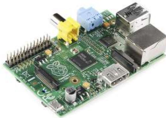
Gambar 2.4 Raspberry Pi Model B
