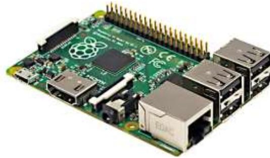
Gambar 2.5 Raspberry Pi Model B+
