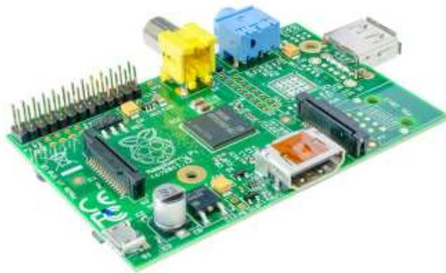
Gambar 2.2 Raspberry Pi Model A
