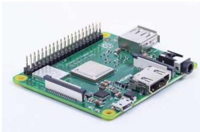
Gambar 2.3 Raspberry Pi Model A+
