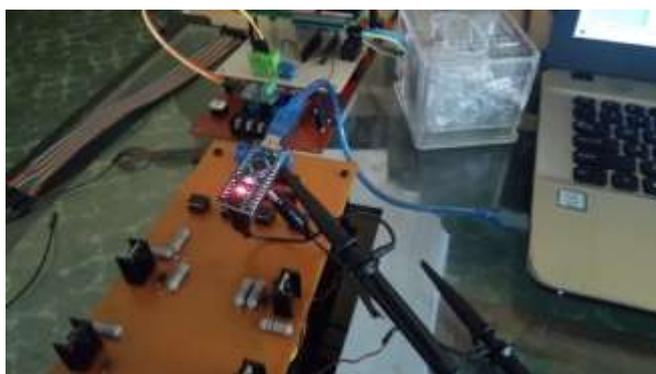
Gambar 3.25 Pengujian *pulse drive circuit*.
