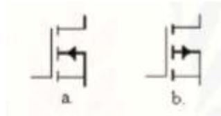
Gambar 2.19 (a). *N-channel enhancement* (b). *P-channel enhancement*
