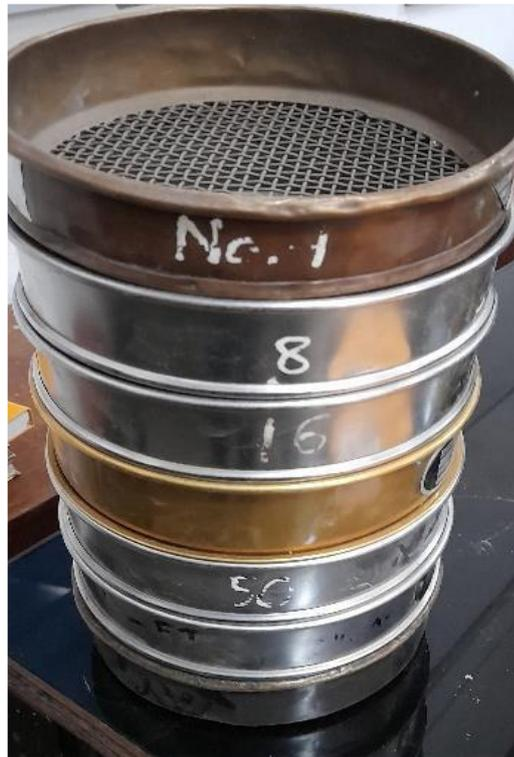
Gambar L-3: Saringan Agregat Halus.
