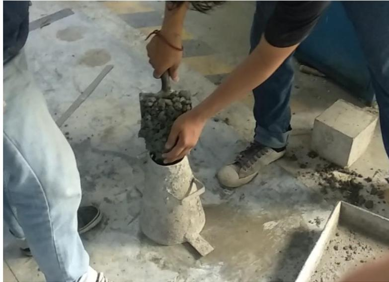
Gambar L-7: Kerucut Abrams.
