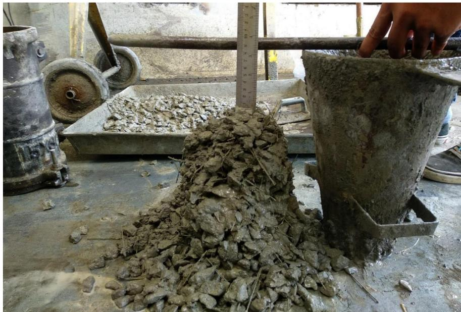
Gambar L-20: Hasil *Slump test*.
