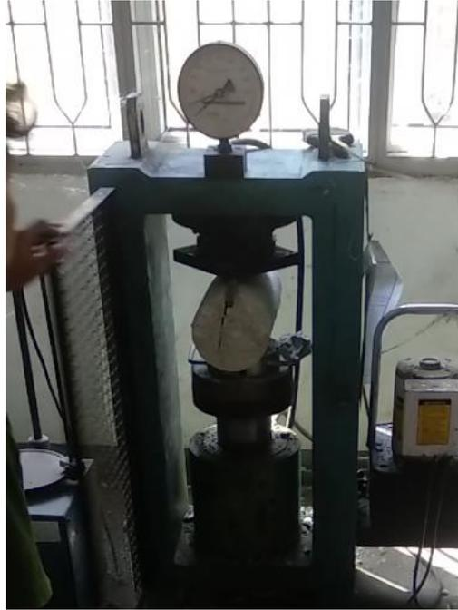
Gambar L-1: *Compressing Test Machine.*
