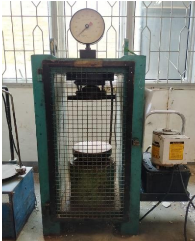
Lampiran 7 : Compressing Test Machine (CTM).
