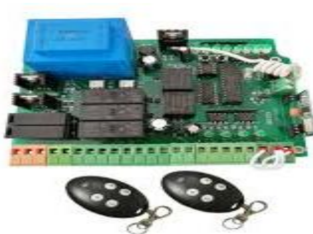
Gambar 2.1.5.Pcb receiver 330mhz dan remot kontrol ( Sumadikarta Istiqomah,2017 )
