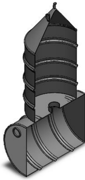
Gambar 3.17 Ketel Tradisional Tampak Section View
