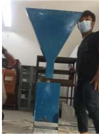
Gambar 3.4: Alat uji V Funnel .
