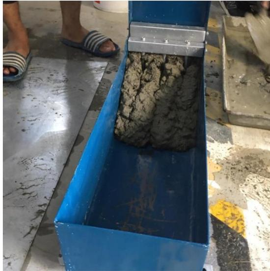
Gambar 3.4 Proses pengujian *passing ability*
