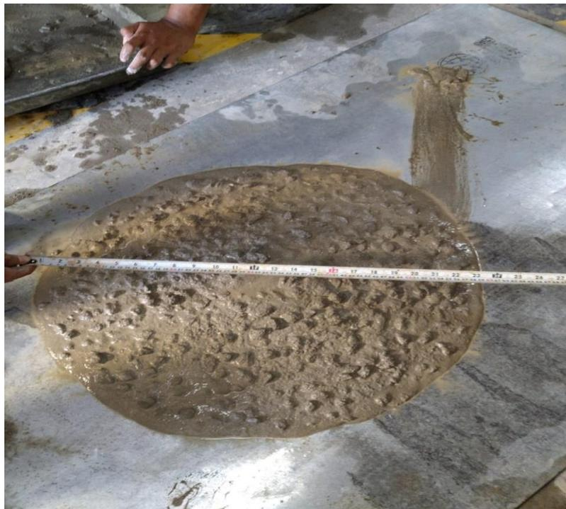
Gambar L.6 Mengukur diameter *Slumpflow*
