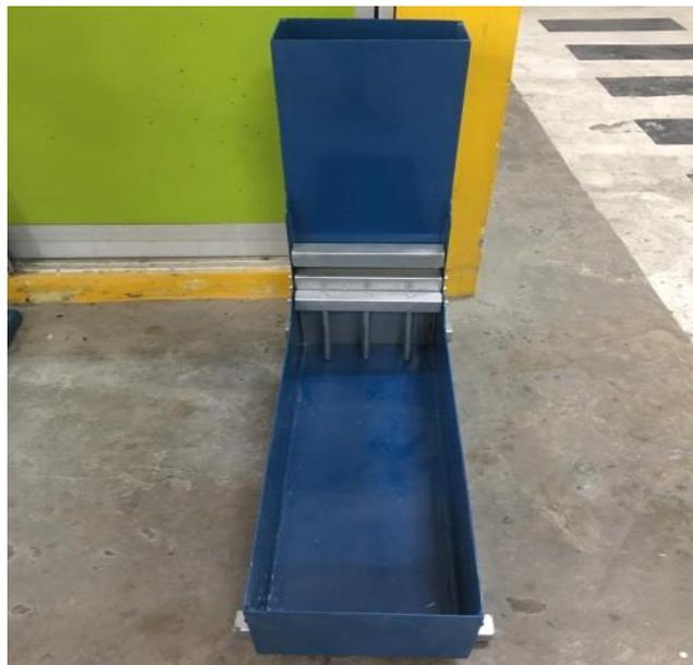
Gambar 2.7 Alat *L-Box Test*
