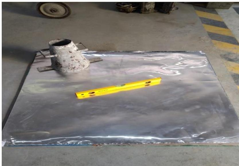
Gambar 2.5 Alat uji *Slumpflow*
