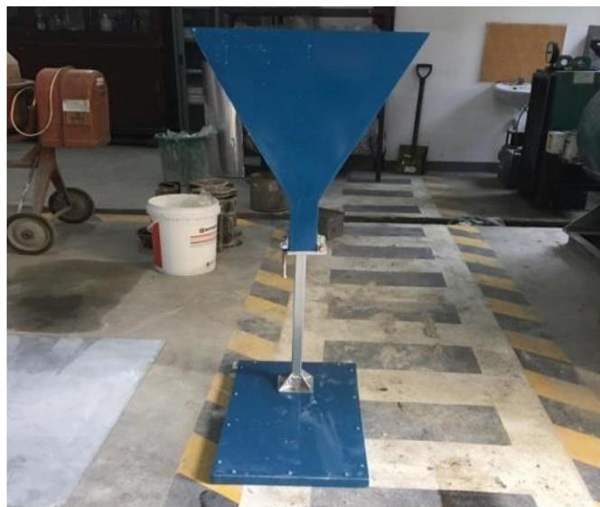
Gambar 2.6 Alat *V-Funnel Test*
