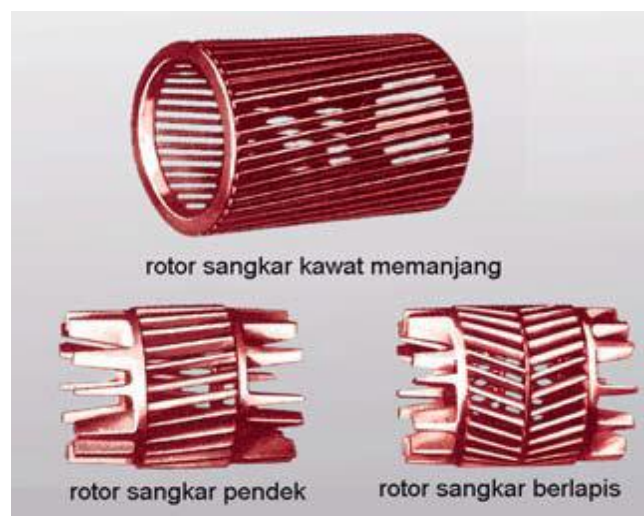
Gambar 2.3 Rotor sangkar ( squirrel cage rotor ).
