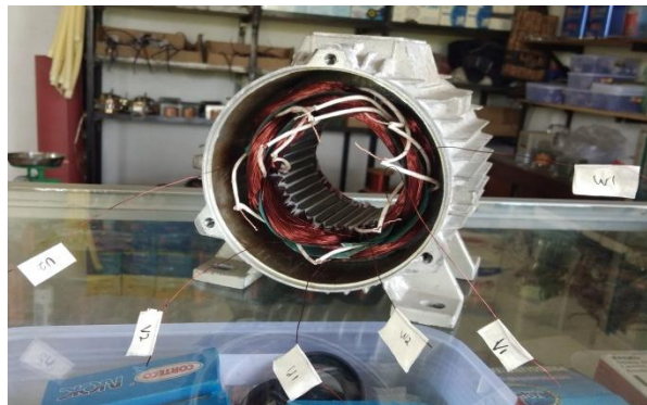
Gambar 4.9 Sambungan belitan stator.
