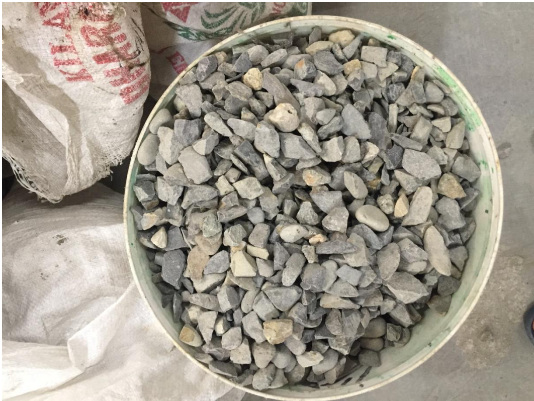
Gambar L.6: Agregat kasar (Ma) \frac{1}{2} inch.
