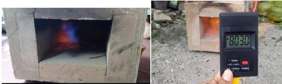
Gambar 3.18 Proses Pemanasan Specimen
