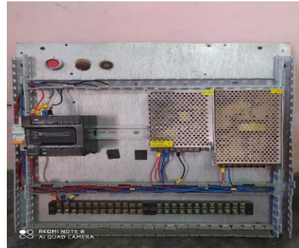
Gambar 4.1. Wiring Power PLC
