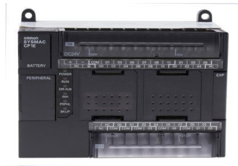
Gambar 2.3 PLC Omron CP1E
