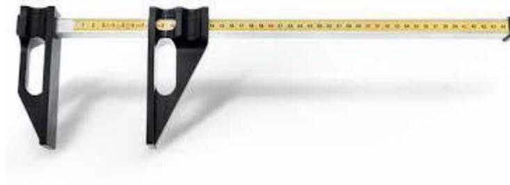
**Gambar 2.2** Sliding Caliper.<sup>10</sup>
