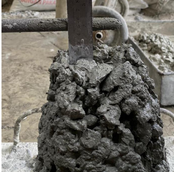
Lampiran 24: Pengujian Slump Test.
