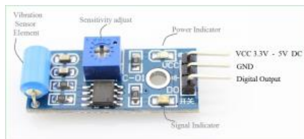
Gambar 2.14. Vibration Sensor SW-420
