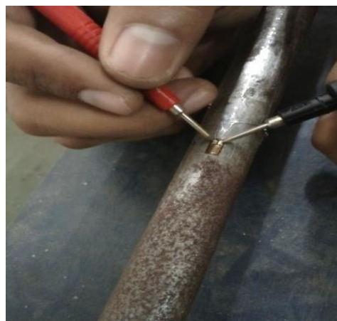
Gambar 4.15 Mengukur tahanan strain gauge
