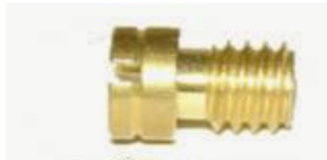
Gambar 2.12: main jet PE, GL-series, Tiger, dsb.
