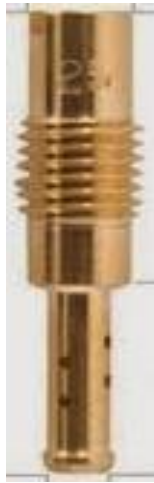
Gambar 2.11: Pilot jet Tiger, GL-series, dsb.
