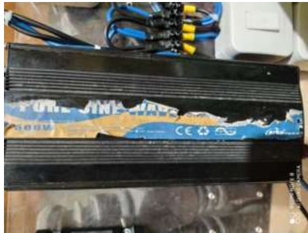
Gambar 2.2 Inverter PSW 500 W
