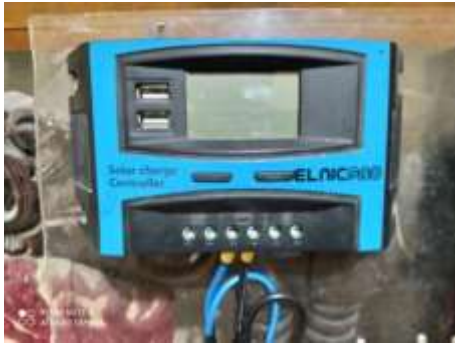
Solar Charging Control 12V 10A
