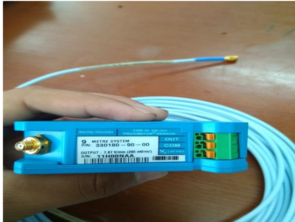
Gambar 2.9 Sensor Proximity Probe Bently Nevada 3300 XL
