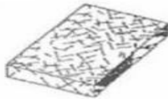
Gambar 2.3 : Discontinuous Fiber Composite(chipped fiber composite) (Van Rijswijk, M.Sc, dkk ,2001)
