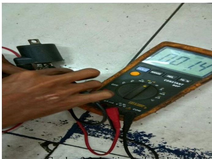
Gambar 3.2: Ignition coil standar (1,4 ohm)
