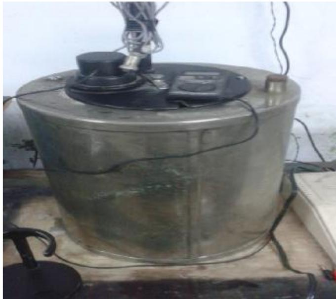
**Gambar 3.33 Kalorimeter Bom**
