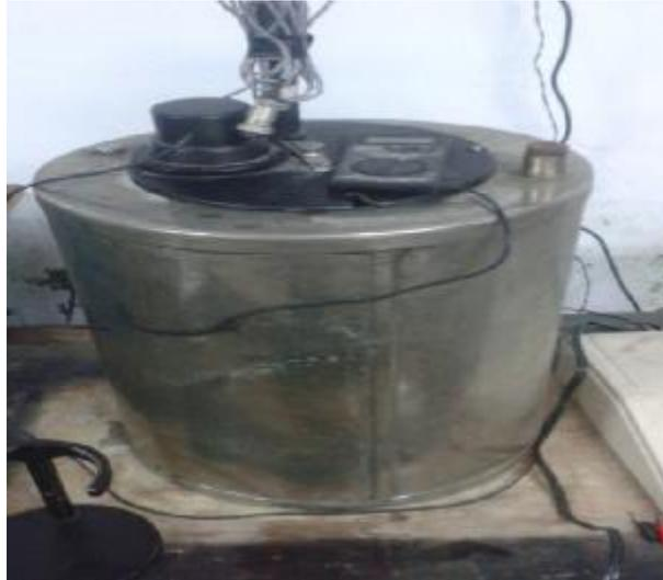
**Gambar 3.24 Kalorimeter Bom**
