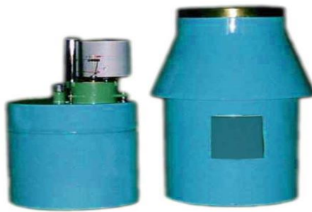
Gambar 2.3: Automatic rain gage.
