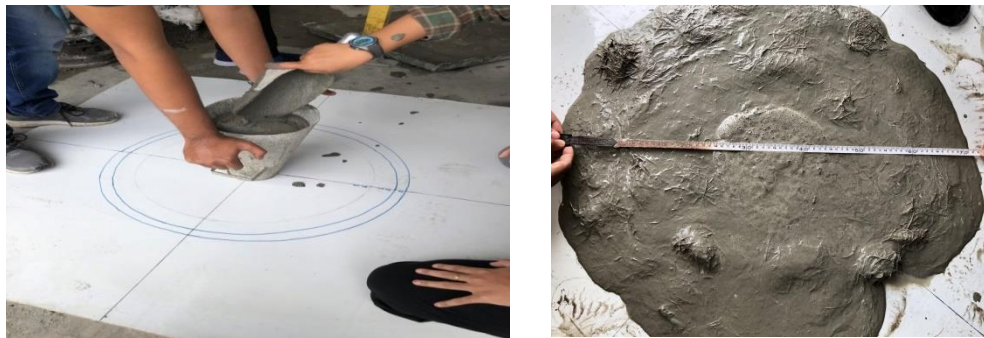
Gambar 3.30 Uji slump flow
