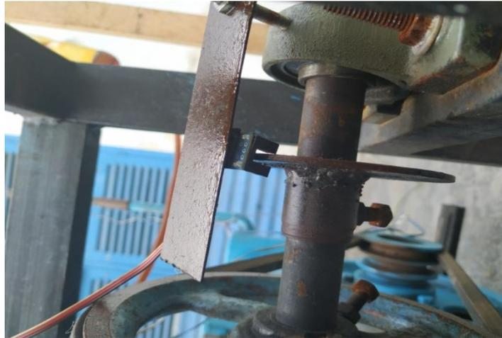
Gambar 3.18. Sensor Putaran ( RPM )
