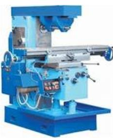
**Gambar 2.1.** Mesin Frais *Horizontal*
