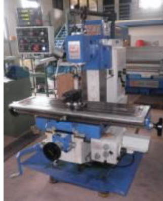
Gambar 2.8. Mesin frais ( milling ) universal Knuth UFM 2 (Romiyadi, 2016)
