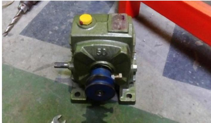
Gambar 3.4 *Gear Reducer*
