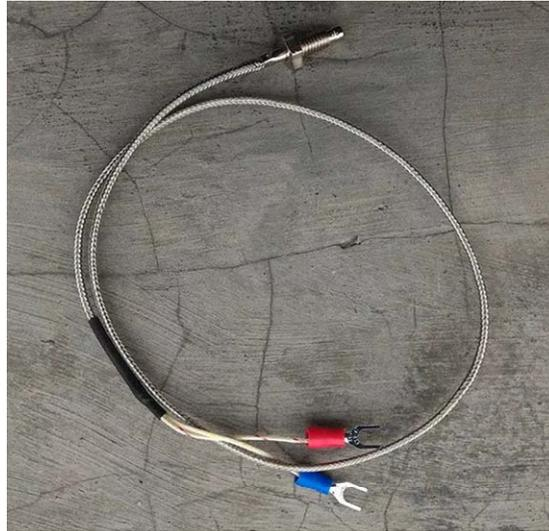
Gambar 3.7 Termokopel (*Thermocouple*)
