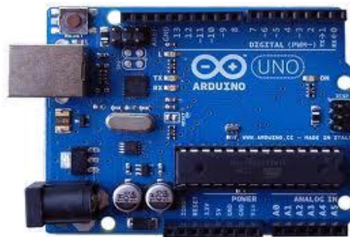
Gambar 2.12 Board Arduino ( Sumber: Yuwono Martha Dinata ; 2015 : 3 )
