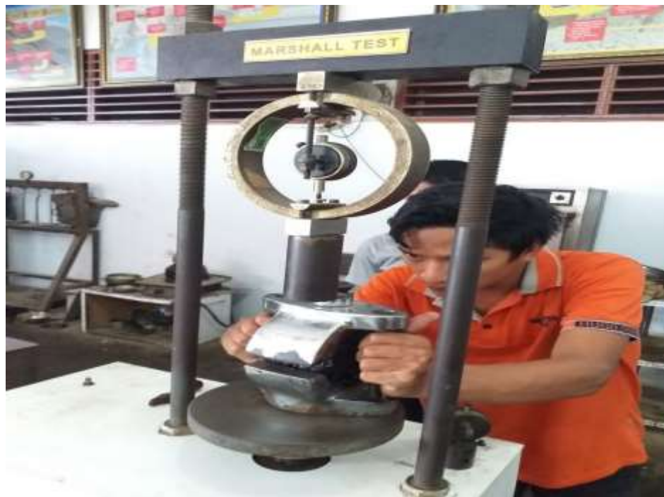
Gambar L10: Pengujian Marshall Test
