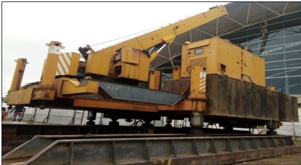
Gambar 2.3: Alat Hydraulic Static Pile Driver (HSPD) Kapasitas 420 Ton.
