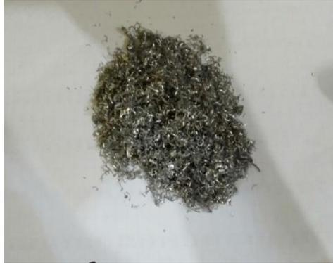
Gambar 3.17. Serbuk Alumunium
