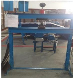
Gambar 3.1. Mesin Press Hidraulik
