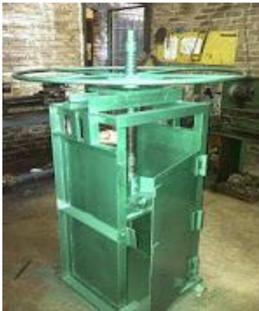
Gambar 2.10 Mesin Pres Tenaga Manual (Remora savalas, 2016)
