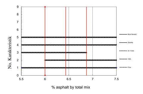
Gambar 4.17: Penentuan rentang (*range*) kadar aspal optimum campuran aspal Penambah serat daun nanas 0,3%.
