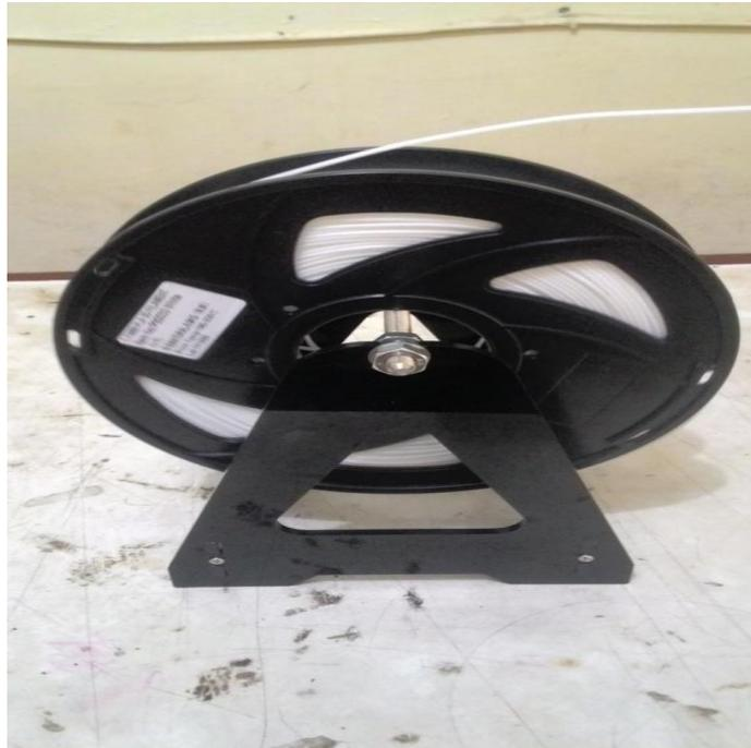
Gambar 3.1 Fillament PLA 3D Printer
