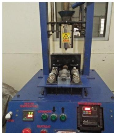
Gambar 3.16. Mesin *Injetion molding*
