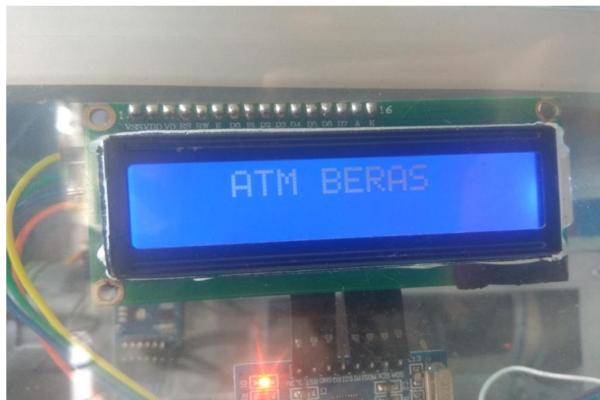
Gambar 2.14 LCD ( Liquid Crystal Display ) 16x2
