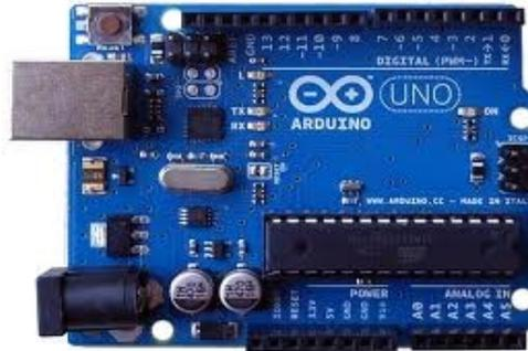
Gambar 2.1. Board Arduino
