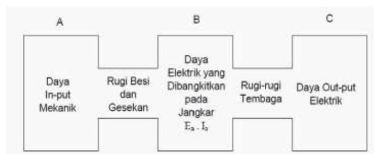
**Gambar 2.31** Diagram Aliran Daya Generator DC
