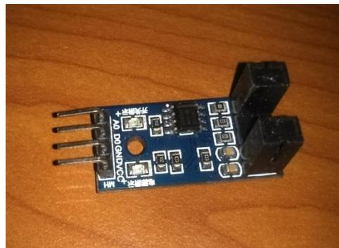
Gambar 3.4 Photo sensor interuptor
