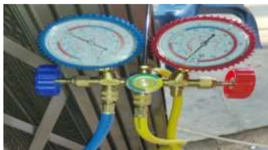
Gambar 3.16 *Manifold Gauge*
