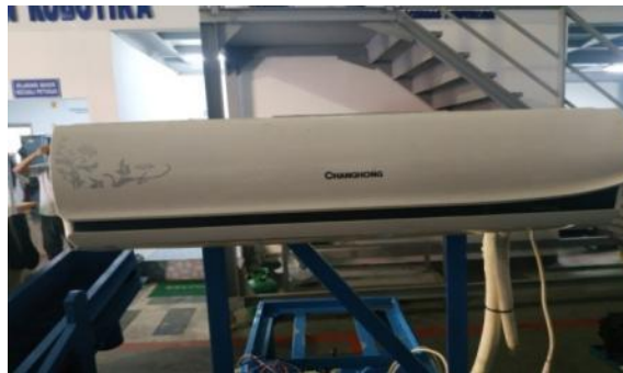
Gambar 3.5 Unit Indoor AC Split
