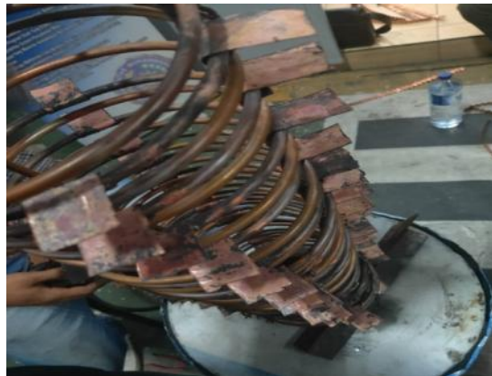
Gambar 4.27. APK Shell Helical Coil Bersirip
