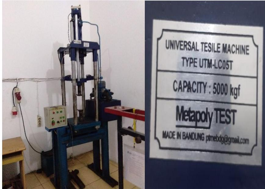
Gambar 3.3 Mesin Uji Tarik (*Universal Testing Machine*)
